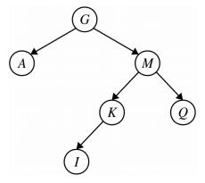
The node M now has two children. To delete M, we start by finding the largest value in its left subtree (K) and replacing M by K. We then delete the node that formerly held K. Since that node has exactly one child, we just replace it with its one child. The result is shown here:
