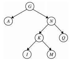
The node N has two children. The largest value in its left subtree is M, so we replace M by N, then delete the node N. This is shown here:
